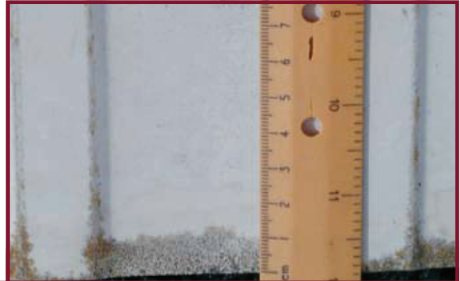
Edge corrosion after 20 years
