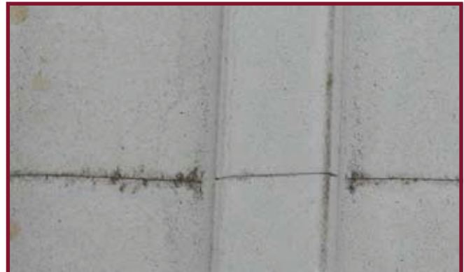
Manufacturer's defect (scribe) corrosion after 20 years
