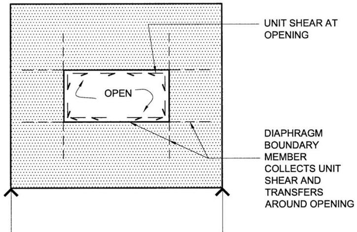
**FIG 4. SHEATHING AND FRAMING DISCONTINUED AT OPENING**
