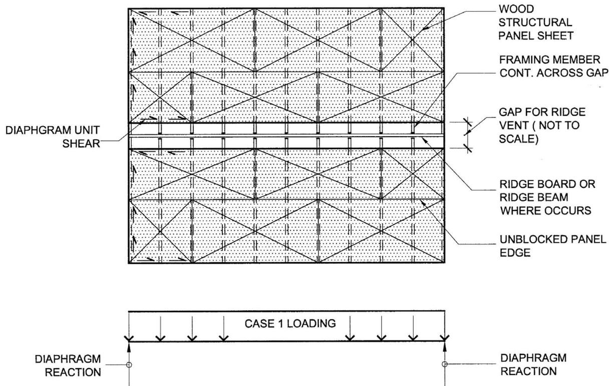
**FIG 1. DIAPHRAGM PLAN VIEW - LOAD DIRECTION 1**
