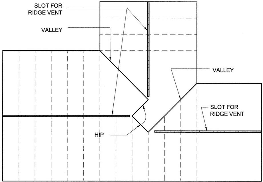
**FIG 3.** ROOF DIAPHRAGM PLAN VIEW - REALISTIC COMPLEXITY
