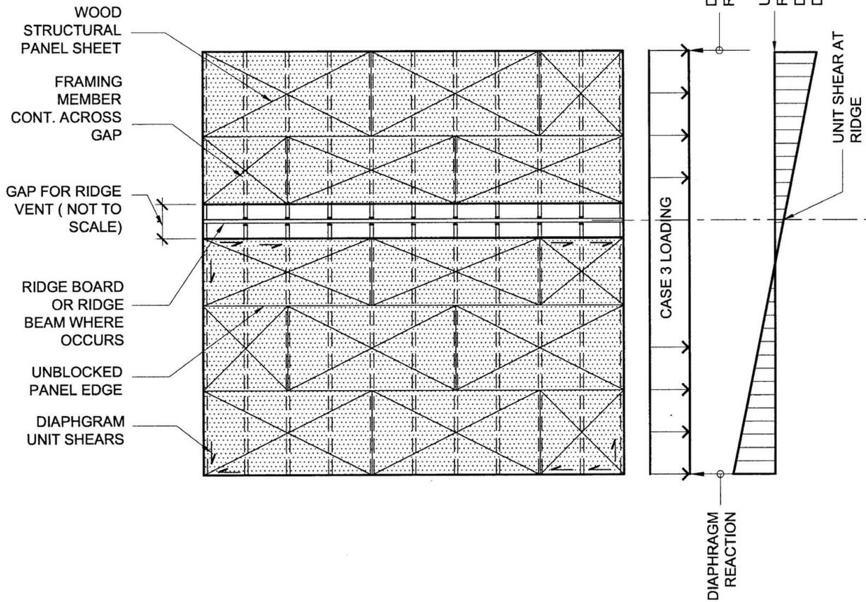
**FIG 2. DIAPHRAGM PLAN VIEW - LOAD DIRECTION 2**
